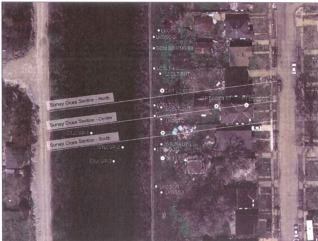
Figure 2.5 – Site Specific Exploration Locations
