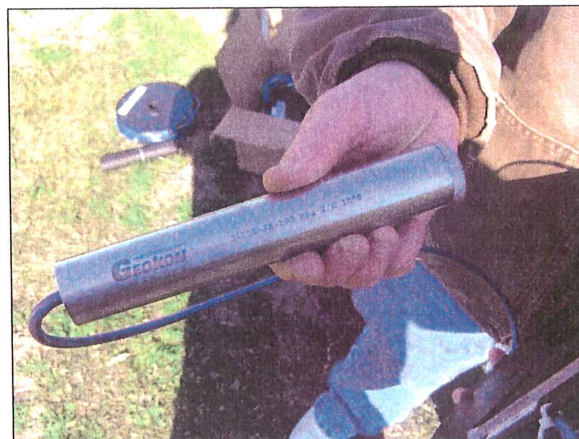
Figure 2.17 – Piezometer Pressure Transducer
