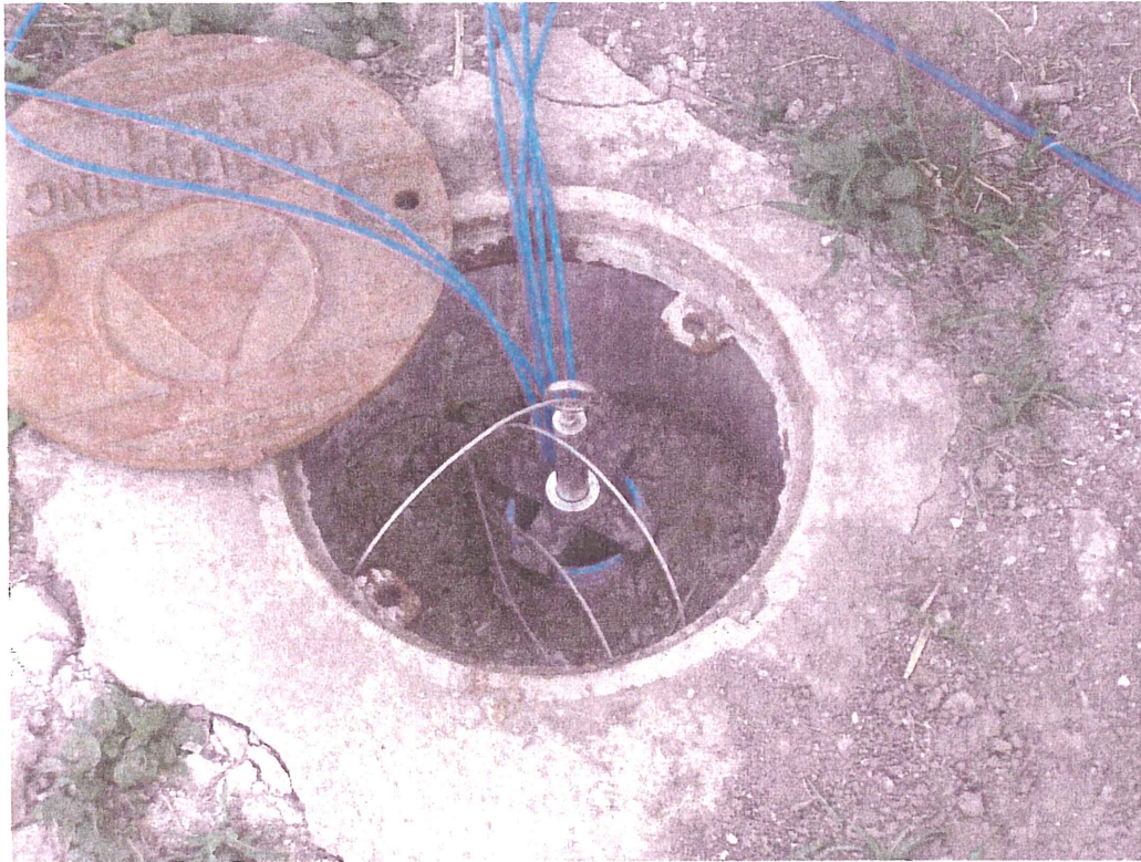
Figure 7.5 - Flush Mount Installation Typical of IPI-2 and IPI-3
